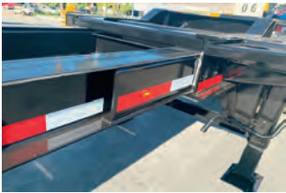
Four C-Channel reinforcements on interior and exterior main beams at the critical gooseneck transition area provides extra strength and durability
