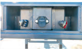
Ease of access & repair of 7-way harness and gladhands
