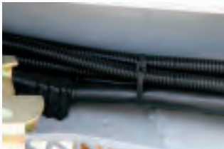
Air and electrical lines protected with automotive wire loom for optimal wire protection
