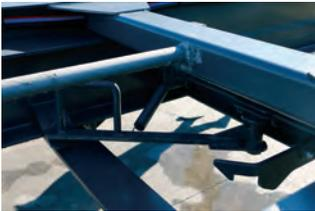
Raised extension actuator lever housed within main beams offers maximum protection from shearing or road hazards
