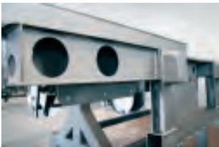
All steel parts are shot-blasted and coated with zinc epoxy primer, before fabrication and after welding
