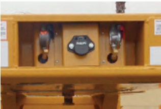
Ease of access & repair of 7-way harness and gladhands
